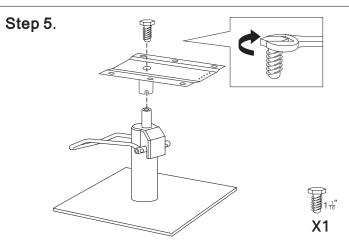
Before moving the chair. You need to make sure the connector Between the chair and the hydraulic pump is Firmly fitted. (Sit on the chair with your body weight Bounce up and down several time until is tight)
